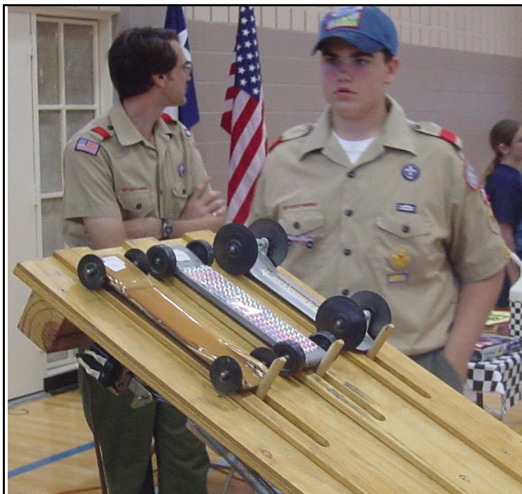
Figure 13 - Cars from the book The Physics of the Pinewood Derby . The center car is also shown in Lecture 4. The left and right cars are pretty fast and have wheels made from regular remolded BSA kit wheels. The times for these cars were predicted closely using the Virtual Race program.
