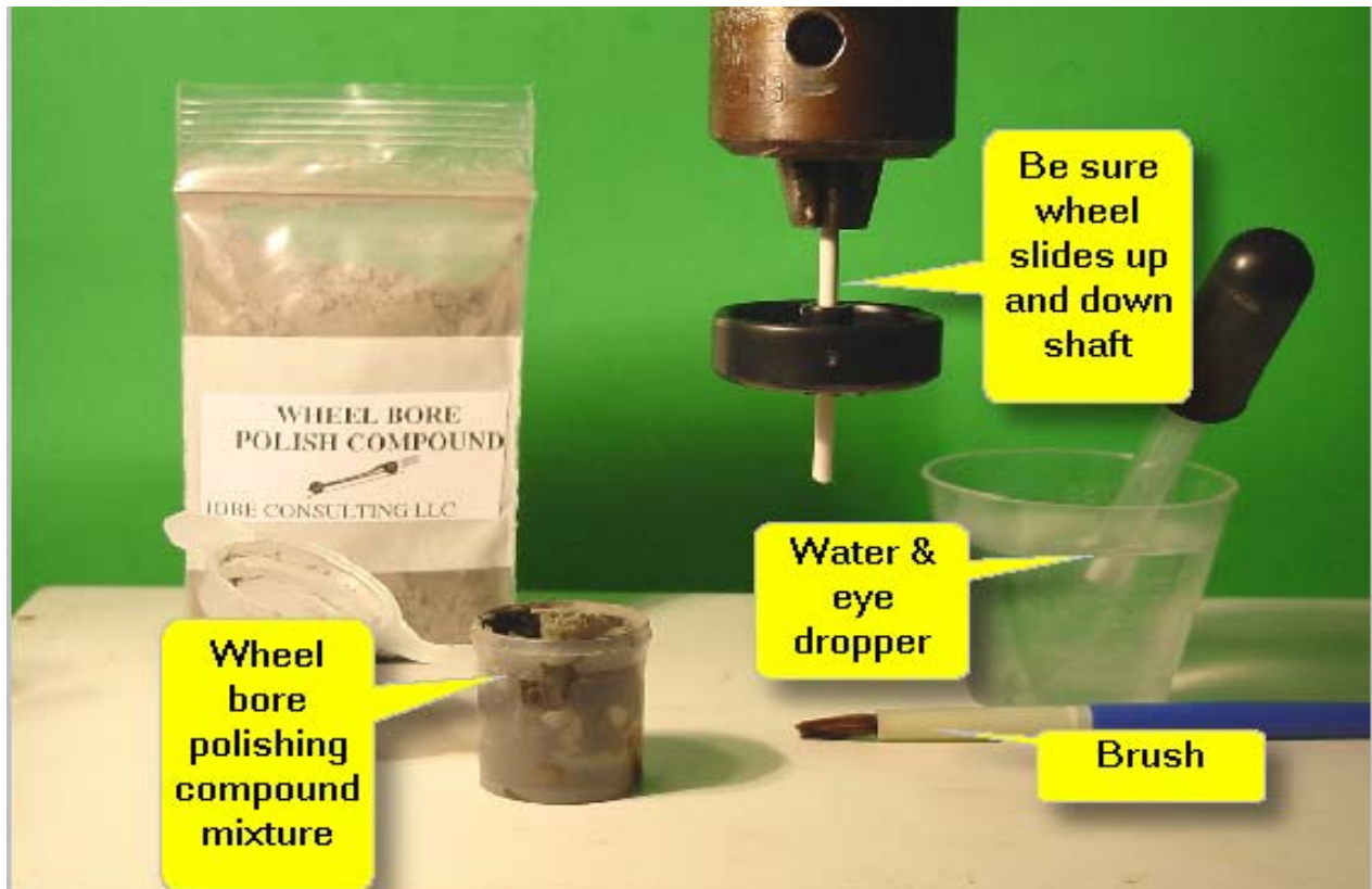
Figure 2 - Getting ready to polish the wheel bore.
