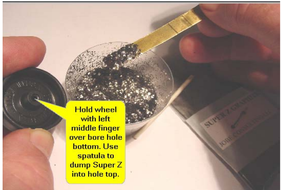
Figure 8 - Using the brass spatula (Grab Bag Item 9) to dip and pour Super Z Graphite into the bore hole.
