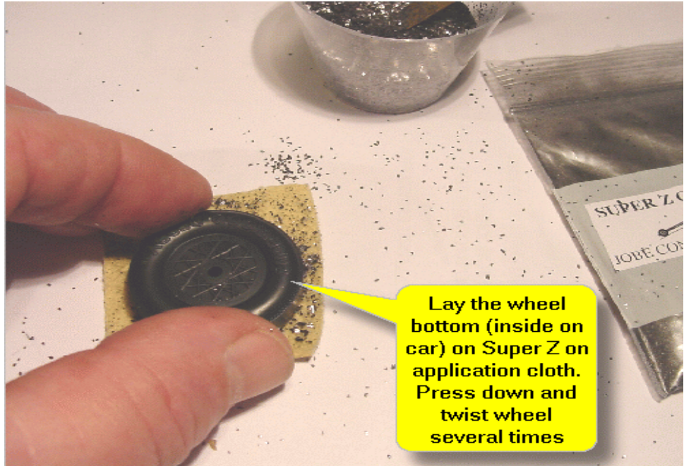
Figure 12 - Rub the inner hub surface on Super Z Graphite.
