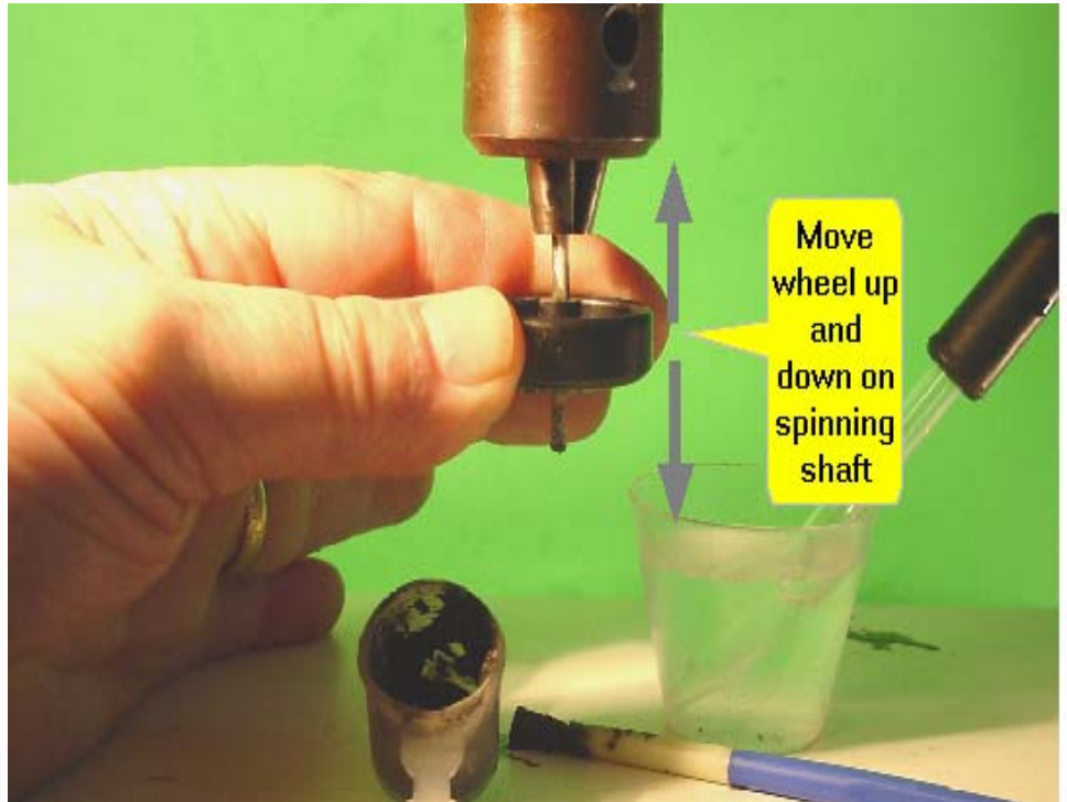
Figure 5 - Move wheel up and down a few times fairly quickly with left hand. ( see video ). You can also paint the shaft above the wheel with the right hand at the same time. Be sure you keep shaft wet with paste as you move wheel. If shaft is not too tight, flip wheel over and take a quick pass through the other side.
