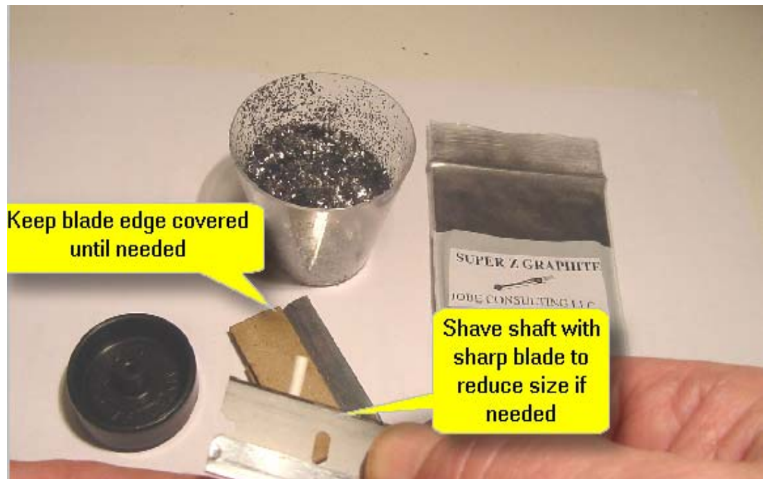
Figure 7 - If a cardboard shaft is slightly too large for the bore, it may be shaved down some with a razor blade (adults only).
