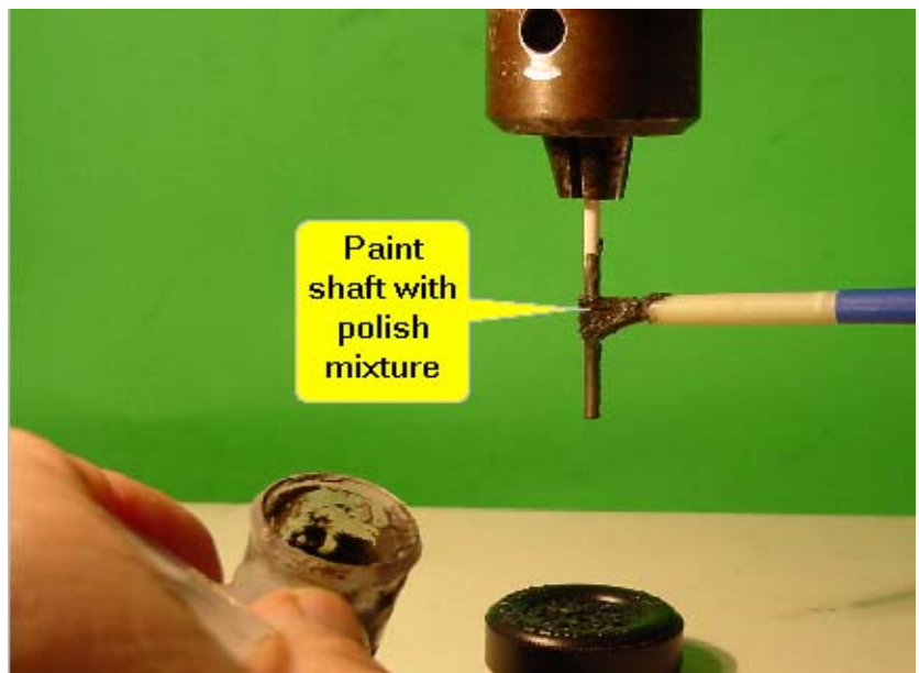
Figure 4 - With shaft chucked in drill, rotate at about 300 rpm while applying bore polish paste with brush.
