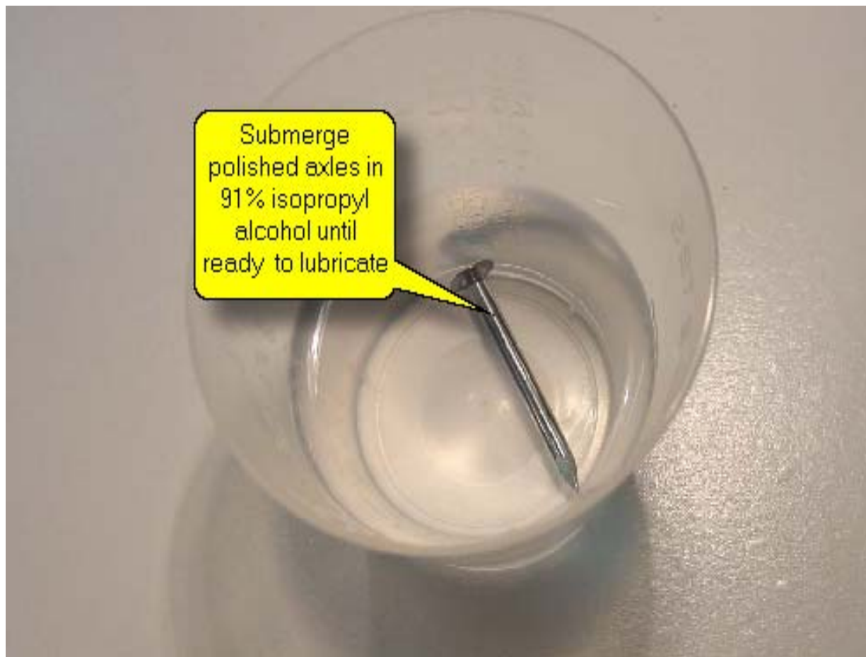
Figure 10 - Keep axle in a small cup of 91% IPA after polishing is complete.
