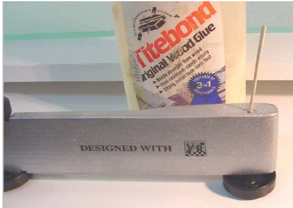
Figure 27 - Adding slight glue to tighten axle hole/axle fit..
