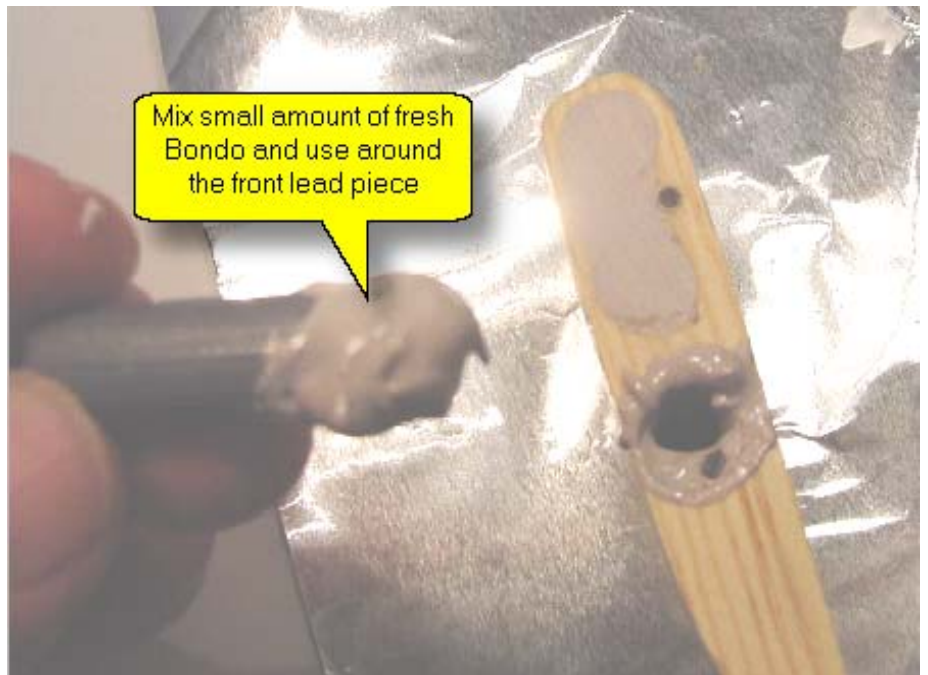
Figure 17 - Using Bondo to secure the front lead piece.
