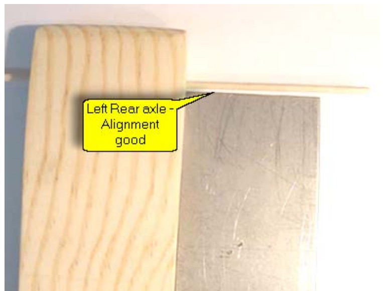
Figure 22 - Checking alignment of left rear.
