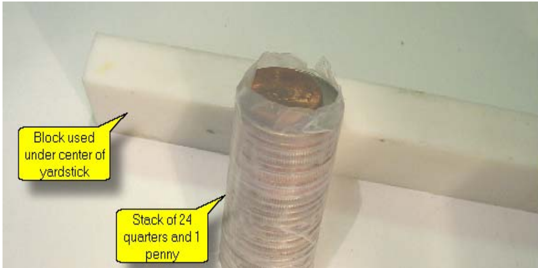
Figure 4 - Tape a roll of 24 quarters together and add one penny to the top of the stack.
